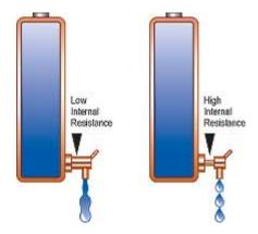
Figure 2: Effects of internal battery resistance. A battery with low internal resistance is able to provide high current on demand. With elevated resistance, the battery voltage collapses and the equipment cuts off.
