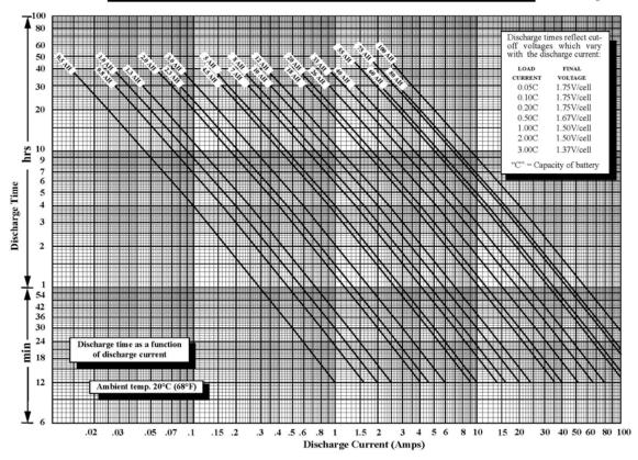
Figure 1, Capacity Variation by Current Load
